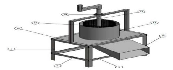
Figure 2: Cad Drawing of the Cassava Sifting Machine
