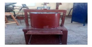
Plate 1: Completed Cassava Shifting Machine
