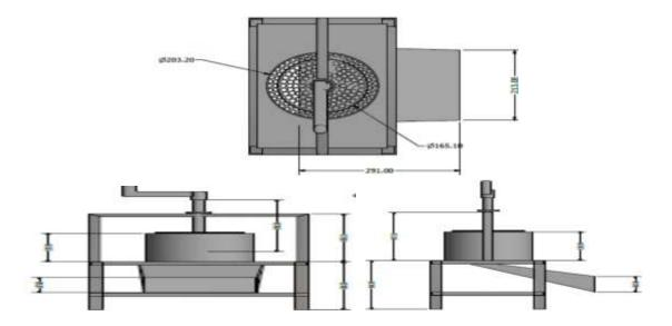
Figure 3: Orthographic Projections of the Cassava Sifting Machine
